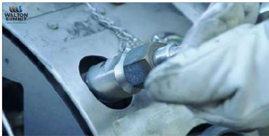
Connect the vent hose to your tank and then remove the filling nozzle from its holder.
