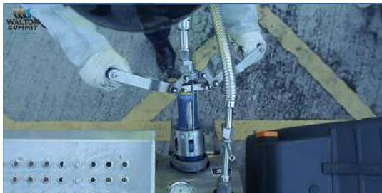
Connect the filling hose by placing the hose on the connection and pushing the handles forward to lock the hose in place.
