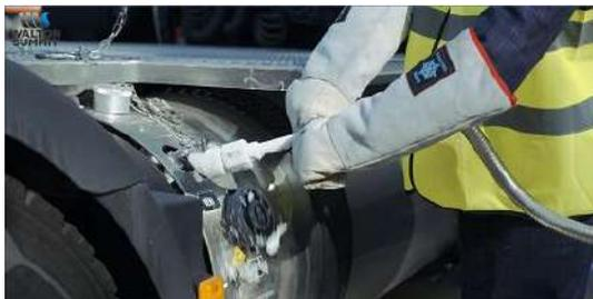
Then remove the vent hose by turning it anti-clockwise and place it back in its holder under the filling hose.
