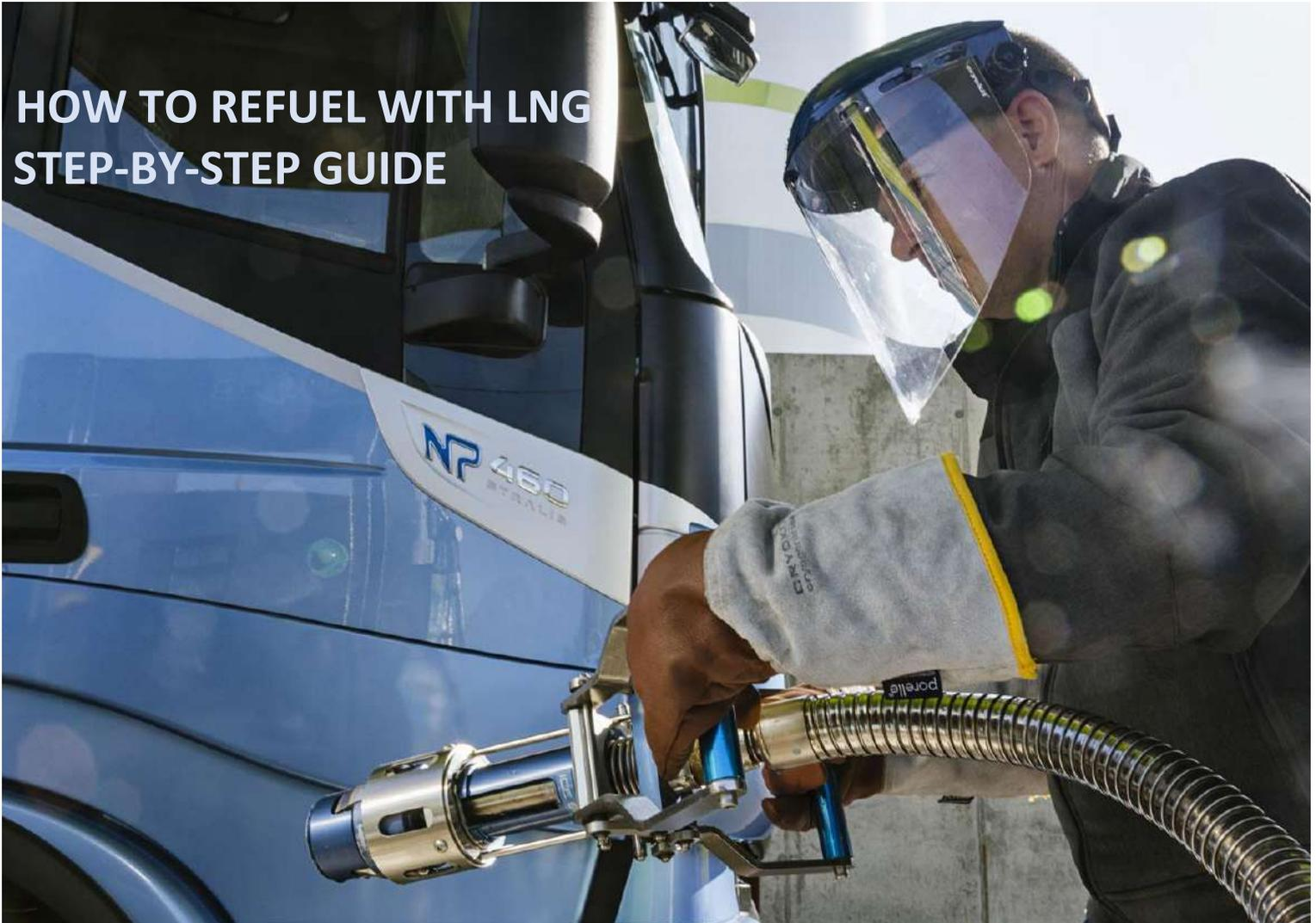
LNG (Liquified Natural Gas) is natural gas the same as you get in your homes that has been super-cooled to  $-162^{\circ}\text{C}$  which has turned into a liquid, so you can store more volume of gas on your vehicle. Below you will see a step-by-step guide on this simple filling process.
