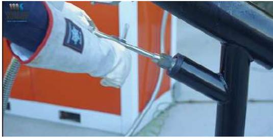
Remove the vent nozzle and use the air hose attached to the filling station to remove any water that has been left from the previous fill around the nozzle and your tank.
