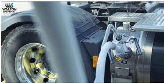
Once the filling has finished the first thing to be disconnected is the filling nozzle which can be released by pulling back the handles.
