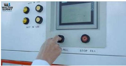
Go back to the main control panel and it will ask you to start filling, press the green start fill button and the filling process will begin.
