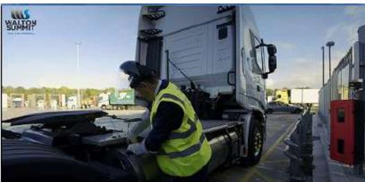
Go to the back of the tank and open and drop down the tank cover and remove the covers from the vent and filling nozzle.
