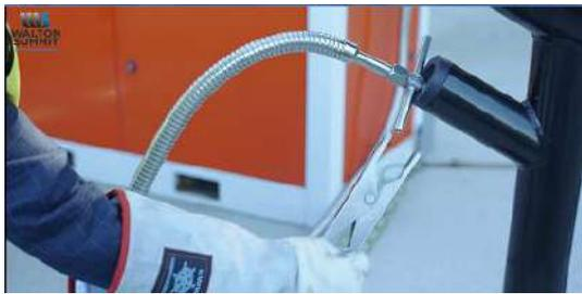
Remove the earth connection from the filling stand and connect this to the bottom of the tank cover (This must be present at all times).
