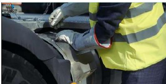
Close your tank cover. If the tank cover is not closed properly the vehicle micro-switch won't let the vehicle start, this is to prevent anyone driving off with any hoses still attached.
